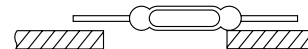
Fig. 7 Precautions to be taken when mounting reed switch on printed wiring board
